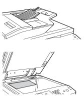
If the X dimension (width) of the document is less than 5-1/2" (140 mm) or the Y dimension (height) is less than 5-1/8" (131 mm), place the original on the document glass. For a thin original, use "Slow Scan Mode".
