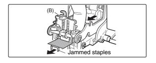
Remove any jammed staples, and then return knob (B) to its original position.
