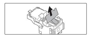
Pull the seal that holds the staples straight out.
