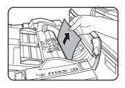
Remove the misfed paper. Be careful not to tear the misfed paper during removal.
