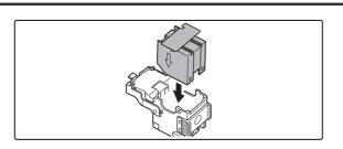
Insert a new staple case into the cartridge. Push the staple case all the way in until it clicks into place.
