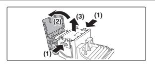
Press the sides from both directions (1) and open the cover in the direction of the arrow (2). Pull the empty staple case straight up and out of the cartridge (3).
