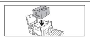
Insert a new staple case into the cartridge. Push the staple case all the way in until it clicks into place.
