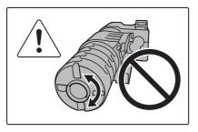
Shake the toner cartridge horizontally. Do not rotate it as shown at left.
