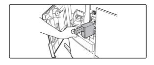
Holding the black handle, slide out the case containing the paper bits, and dispose of them properly.
