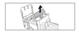
Pull the seal that holds the staples straight out.
