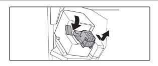
Lower the blue lever in the stapler and slide out the staple cartridge.
