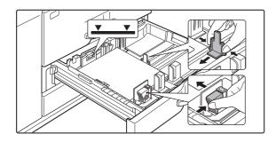
Adjust the guide plates A and B by squeezing their lock levers and sliding them to the paper size to be loaded.
