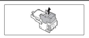
Pull the empty staple case straight up and out of the cartridge.
