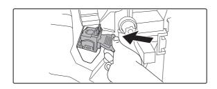
Put the staple cartridge back into the stapler.
