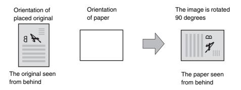
This function operates in both auto paper selection mode and auto image mode. Rotation can be disabled using "Rotation Copy Setting" in the System Settings (Administrator).
