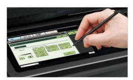
High-resolution touch-screen with stylus pen for easy point-and-touch operation.
